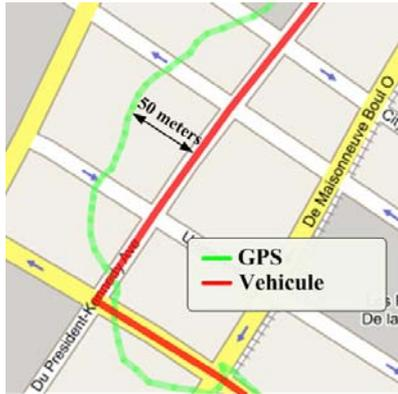
Figure 8. GPS positioning error in dense urban environment
