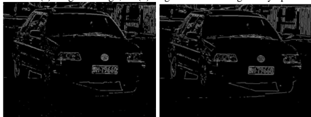
(c) Edge detection by Roberts operator (d) Edge detection by Sobel operator
