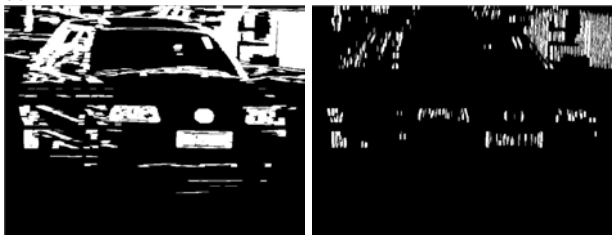
(a) Horizontal dilation operation; (b) The result of opening operation Figure 7. The results after using different processing methods
