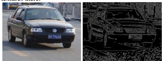
(a) Original image; (b) Edge detection using Canny operator
