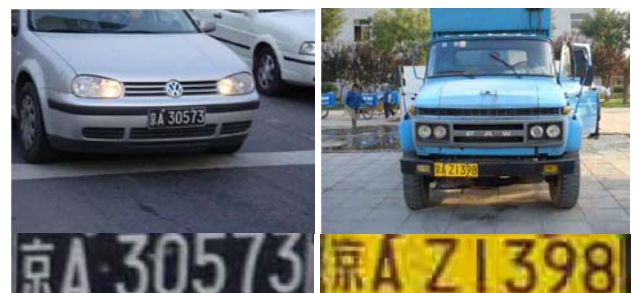
(c) The location result of the license plate influenced heavily by headlights (d) The location result of the license plate whose words are black
