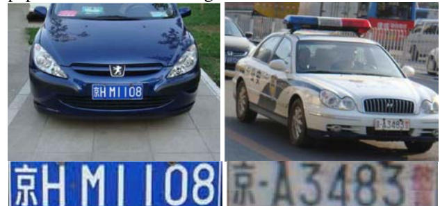
(a) The location result of the license plate whose background has the same color with the vehicle (b) The location result of the license plate influenced by vertical textures of the radiator
