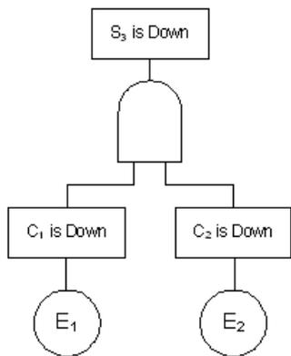
Figure 2. Classical fault tree model of parallel components
