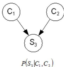
Figure 3. Equivalent Bayesian Network of parallel structure
