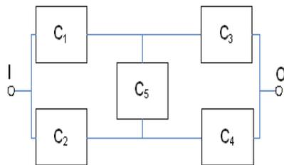
Figure 5. Reliability diagram of the bridge system.
