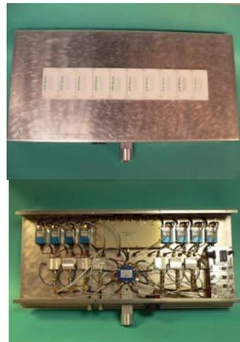
Figure 5. Eight elements ULA array receiver.
