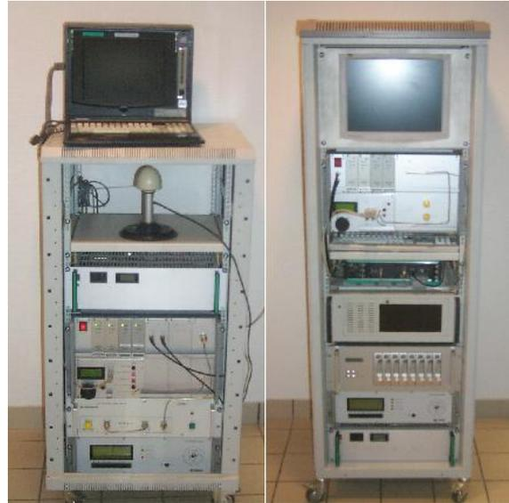
Figure 1. MIMO channel sounder transmitter and receiver.
